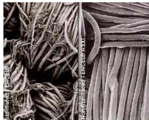
As suggested by the photo, the tendency to fibrillate can be controlled during manufacturing. (Tencel is the normal lyocell and Tencel A100 is the non-fibrillated product.)
