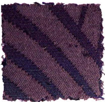
At the same time, many of these manufacturers will not warranty their products for color changes or long-term damage. The darker colored fabric (below left) is the untreated fabric, while the sample directly below has been FR-treated.
